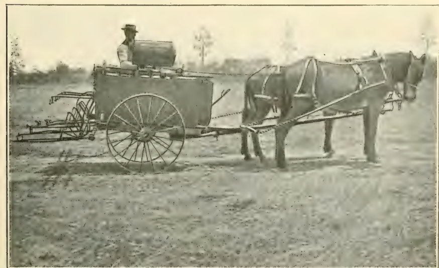
FIG. 217.—Field sprayer, with modifications, adapted for potato spraying, by L. C. Corbett, operating at the Virginia Truck Experiment Station, Norfolk, Va.
